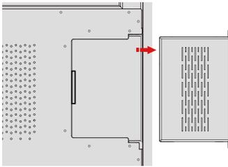
Step 2: Push the internal PC into the internal PC port at the rear of the screen from right to left.
